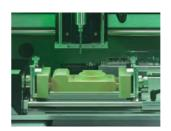
Optional Rotary Axis with self-centering headstock and tailstock workpiece clamps.
