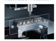
The MDX-50 features a 5-station Automatic Tool Changer with an auto-sensing function to detect tool length and ensure milling accuracy.
